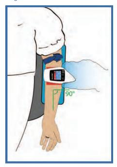
The AV300 should be positioned at an approximate 90° right angle (perpendicular) to the direction the vein flows or is expected to flow. You can then often improve display quality by changing this angle slightly.
