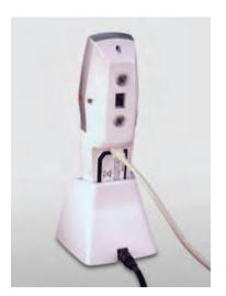
Plug the USB cable into the AV300's USB port, which is above the battery, and place the AV300 in its charging cradle. Plug the other end of the USB cable into your PC's USB port. Then start the AV300 PC application, which begins looking for the attached AV300. Be sure to leave the AV300 in its charging cradle while it's plugged into the computer. The AV300 fits in the cradle with the battery cover removed.
