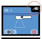
When the AV300 is placed into a powered stand, a tone sounds and the battery indicator changes to a plug, indicating that the AV300 does not require battery power. During this time, the AV300's battery is also being charged.
